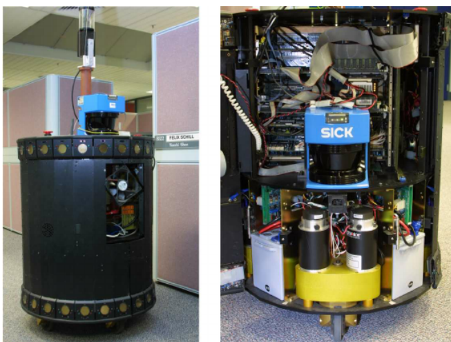
Fig. 4: Four Castor Wheels with eight motors - Nomad 4
