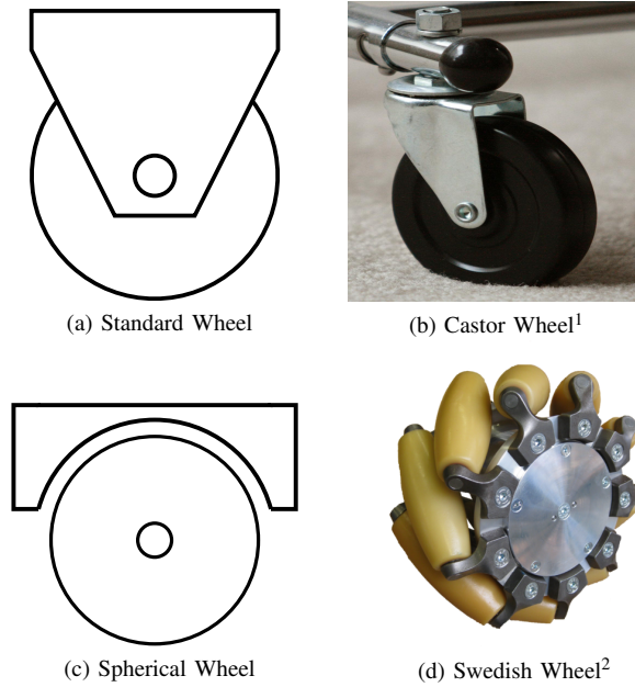
Fig. 2: Four most common wheel types
