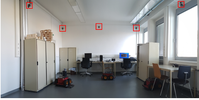
Fig. 7: Case studies laboratory, IR-cameras indicated in red.
