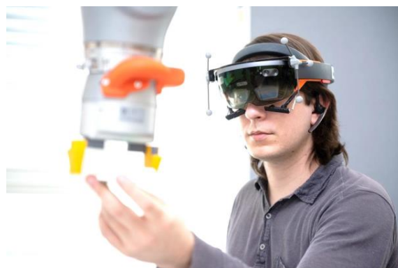
Figure 1: Human-robot collaboration and intuitive interface (HoloLens, eye tracking, markers for OptiTrack localization) for the assessment of human factors state to characterize key features in the collaboration domain.
