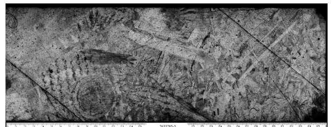
Fig. 1. Footwear impression(s) from a real crime scene collected using a gelatin foil lifter.
